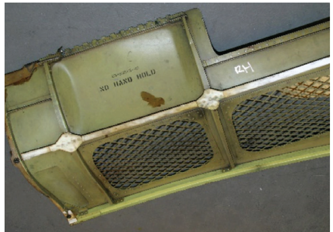
Figure 9: GORE® SKYFLEX® Aerospace Tapes, 700 Series installed on engine access door.
