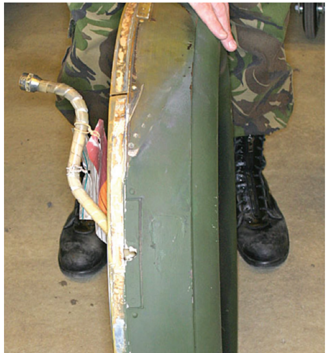
Figure 4: Chafing damage to engine inlet D-ring cowling at mating surface.
