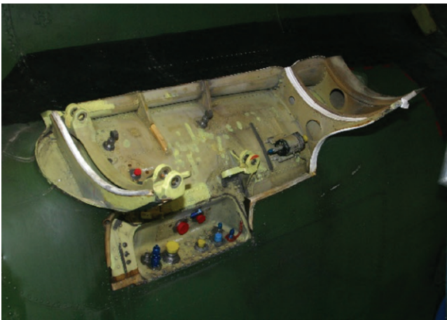
Figure 8: GORE® SKYFLEX® Aerospace Tapes, 700 Series installed on engine mount structure.
