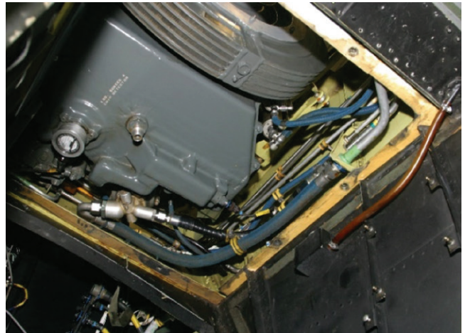
Figure 16: GORE® SKYFLEX® Aerospace Tapes, 700 Series applied to mounting surface for forward transmission drip pan.
